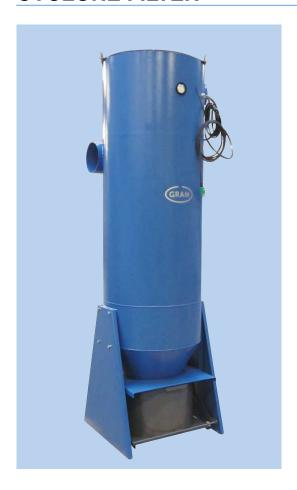
Compact compressed-air cleaned filter unit with timer control for filtration of welding smoke, grinding dust, cutting smoke and dusty air containing metal, rock, plastic etc. or from handling various powder mixes.
