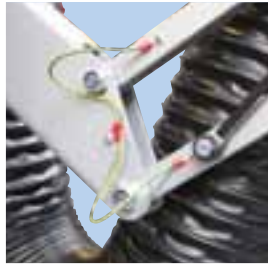
Bend Bend bottom with earth cable connections to parallelogram.
